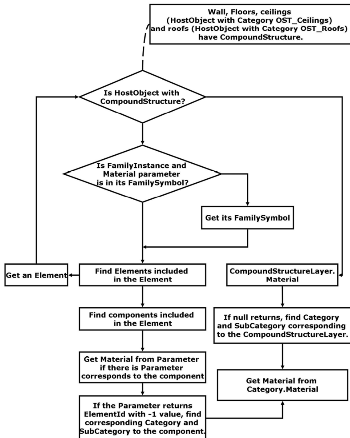
Figure 110: Getting Element Material workflow
