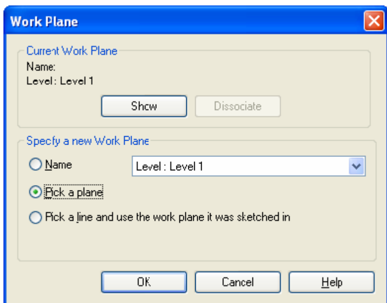
Figure 77: Pick a Plane to identify a new Work Plane
