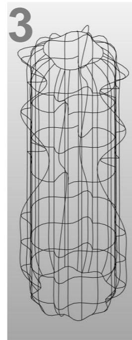
24 Mullion Splines interpolating Floor Plate Control Points
